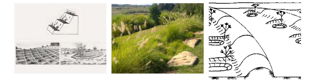
Bioswales can be improved by a chain of ponds or rock barriers to slow the water down. More water retention.
